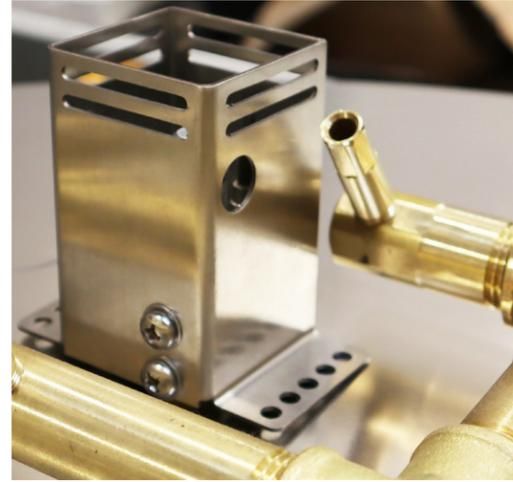
Photo 4b: Pilot Hood Circular Opening Positioning
