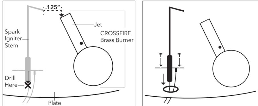
If the distance to the jet is greater than .125", you can adjust the position by **gently** bending the spark ignitor by the stem. Bending too far can result in breakage. Do not flex at the existing bend, this can result in breakage. If the spark ignitor is too far away or too close to the jet, you will not get a strong enough spark to light the burner.
