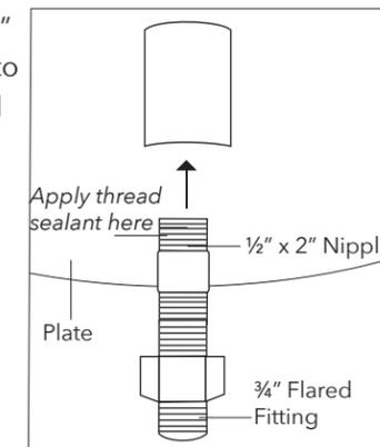
**4. LOCATE 2ND FLARED FITTING AND CONNECT TO KEY VALVE**
