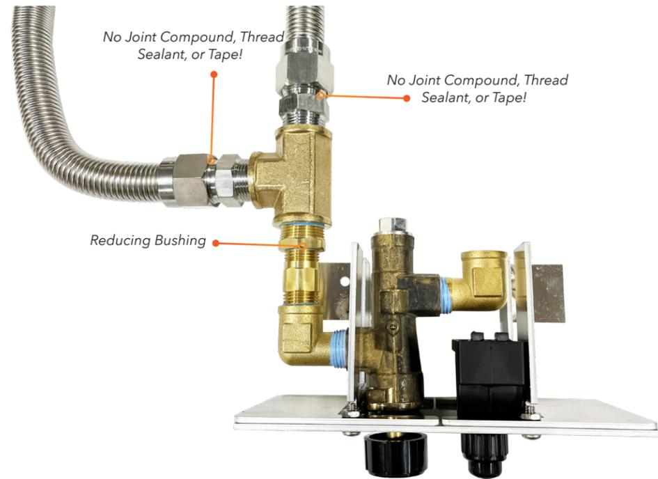
Photo 12: Final Assembly with Flex Lines Connected
