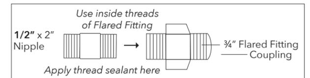
Then, connect the 1/2" x 2" Nipple fitting into the coupling located on the bottom of the aluminum plate. Tighten.
