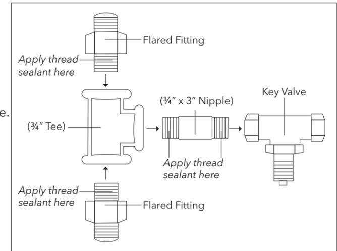
**7. CONNECT FLEX LINES TO COUPLING AND KEY VALVE CONNECTION**
