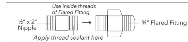
Then, connect the 1/2" x 2" Nipple to Gas Valve.
