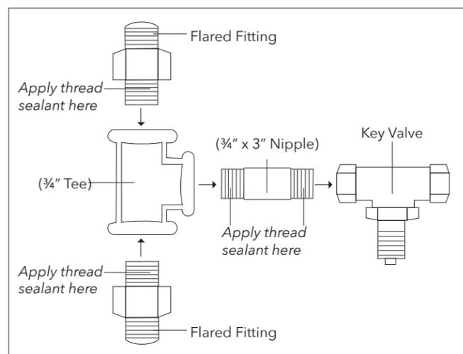
**6. CONNECT FLEX LINES TO COUPLING AND KEY VALVE CONNECTION**
