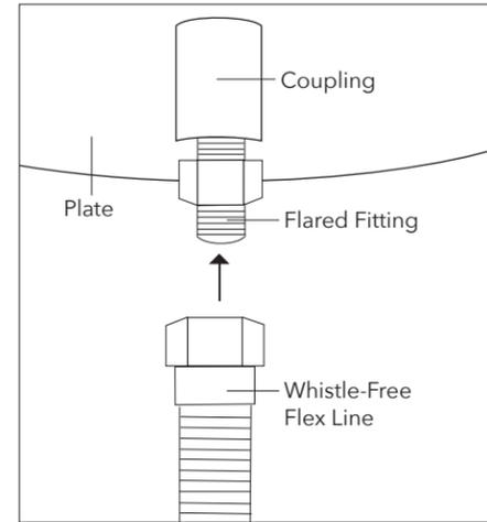
**5. LOCATE 2ND FLARED FITTING AND CONNECT TO KEY VALVE**
