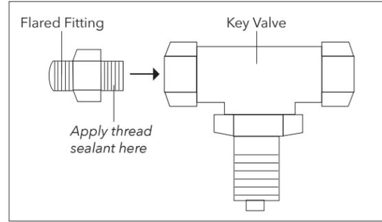
**5. CONNECT FLEX LINE TO IGNITION AND KEY VALVE**
