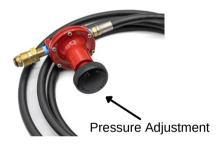
3. Turn the adjustment knob counter-clockwise 3-5 full rotations to decrease the pressure before lighting the fire
